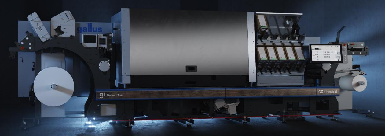
1200 x 1200 dpi | CMYK (up to 88 % PANTONE®) | White 85 % opacity (70 m/min) | 340 mm printing width | Productivity 1428 m²/h drop freeze pinning | automatic cleaning | inkjet control - vision system | CO2 - neutral
